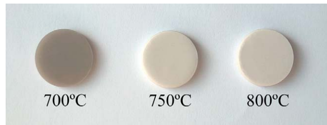
Fig. 5. Appearance of glass–powder compacts made of composition 1 after heat treatment at different temperatures for 1 h.
